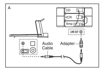
B. Plug one end of the audio cable into the jack on the front of the treadmill near the power cord. Plug the other end of the cable into the included adapter. Plug the adapter into an RCA Y-adapter (available at electronics stores). Next, remove the wire that is currently plugged into the LINE OUT jack on your stereo and plug the wire into the unused side of the RCA Y-adapter. Plug the RCA Y-adapter into the LINE OUT jack on your stereo.
